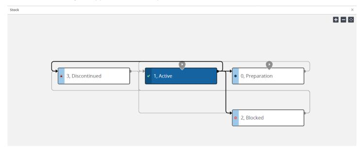
Refer to the following table, for a description of the components of the status flow diagram.
